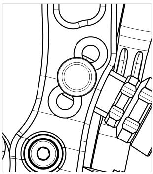
You can adjust stiffness of the throttle pedal by choosing one of three positions on the throttle pedal arm. Unteighten preload nut to remove spring compression. Take Magnetic Quick Pin out of the socket and move it to a different position. Pay attention to the throttle spring assembly rod end bearing so it won't fall out of the pocket.
