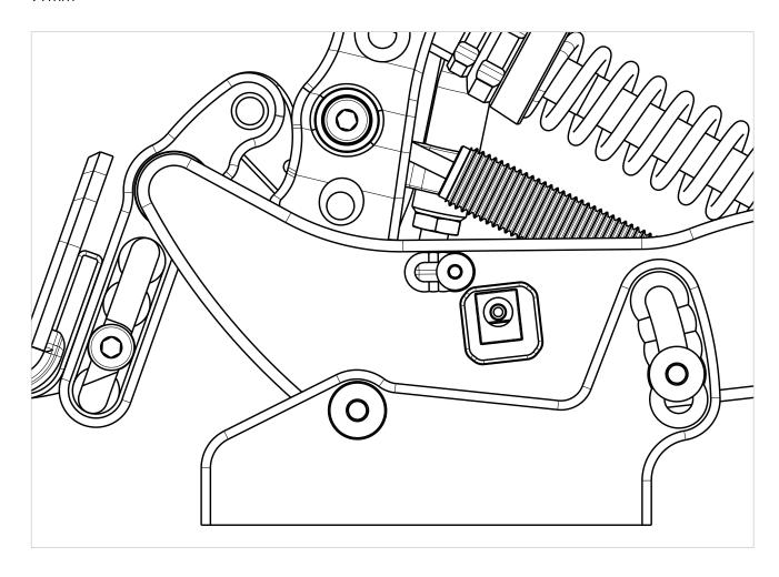
Tighten the M4 bolt so it doesn't slide when the pedal is pressed.
