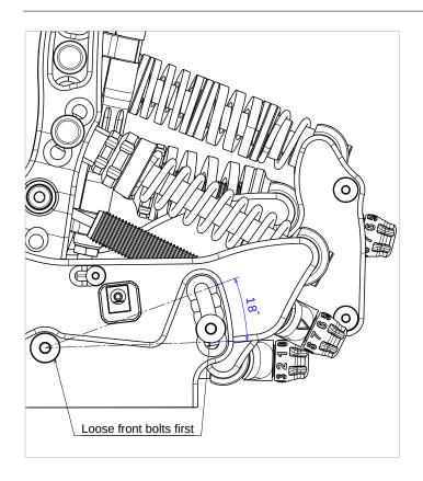
The PurrPRO FORMULA PEDALS mounted on the sim rig offer the ability to adjust the whole pedal angle within 18 degree range. To adjust the pedal angle you will need to lose front two bolts to allow a degree of freedom for axis of rotation and loose rear two bolts to make adjustment possible.
