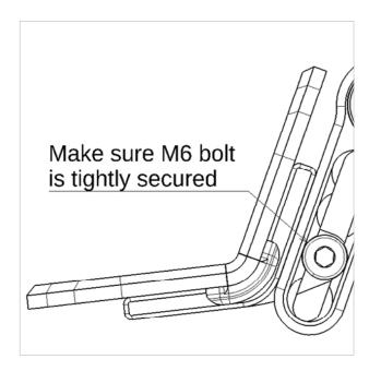
Be aware that M6 bolts holding A.H.S assembly have light threadlock applied - we recommend Loctite 222.
