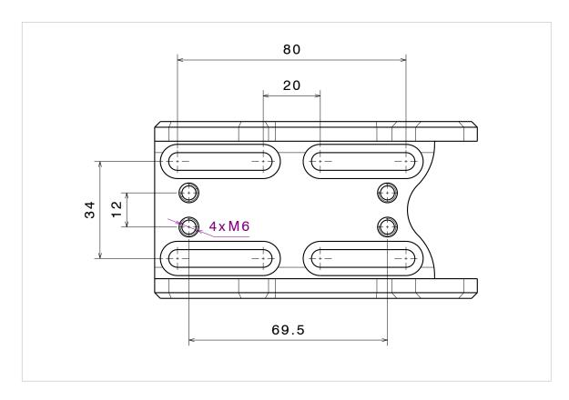
Recommended M6 bolts torque is 11Nm. After securely tightening all bolts, pedals are ready for operation.
